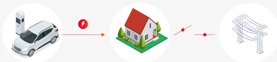
Figure 4. Islanded V2B Operation During Grid Outage
